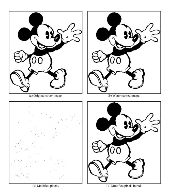
**Figure 3:** A 295×331 image reversibly watermarked with 128-bits MAC, using 496 pixels to store the payload.
