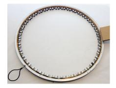
Fig. 1. Prototype of the "hula hoop" scanner. We mounted 36 ultra-sound distance measuring sensors at the inner side of a bicycle rim. At right, there is a board with auxiliary circuitry and connectors to the Arduino.
