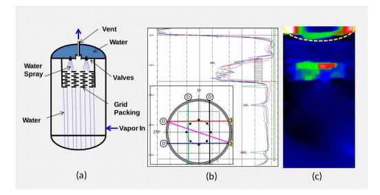
Figure 7: Desaerador sketch (a), conventional gamma scan orientation and plot (b), density profile obtained by tomographic gamma scan (c).
