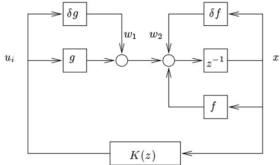
FIG. 3.2. Block diagram representation of the perturbed state-equation.
