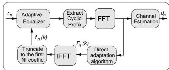
Fig. 4. Combined use of channel estimation and time equalization.
