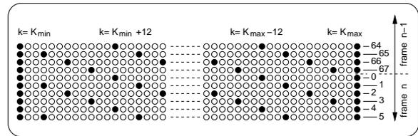
Fig. 2. Typical pilot carrier distribution pattern of DVB-T.
