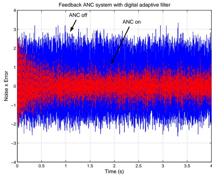
Figure 6: Feedback ANC system with digital adaptive filter without (solid line) and with (dashed line) using the ANC system
