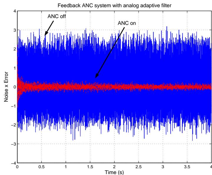
Figure 7: Feedback ANC system with analog adaptive filter without (solid line) and with (dashed line) using the ANC system
