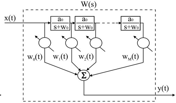
Figure 4: Analog adaptive filter
