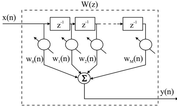
Figure 3: Digital adaptive filter
