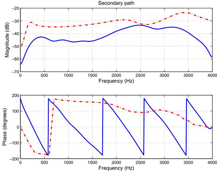
Figure 5: Digital secondary path (solid line) and analog secondary path (dashed line)
