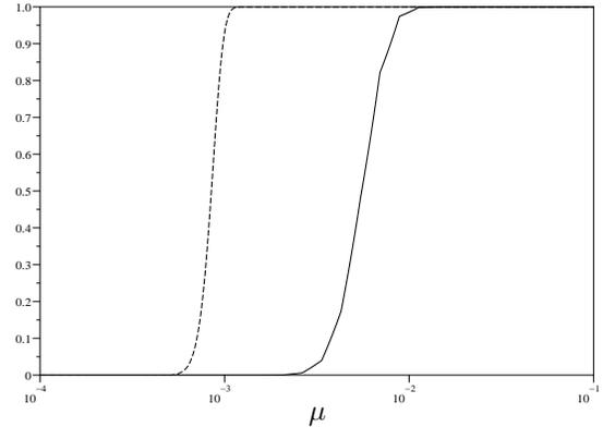
**Fig. 2.** Probability of divergence for LMF, iid regressors, uniform noise,  $M = 100$ ,  $\sigma_0^2 = 0.01$ . Dark curve: observed probability in  $10^5$  runs with 100 time-steps. Broken curve:  $P_d$ .
