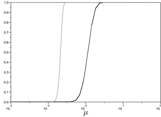
**Fig. 4.** Probability of divergence for LMMN, tap-delay line regressors, Gaussian noise,  $M = 100$ ,  $\sigma_0^2 = 0.01$ ,  $\delta = 0.8$ . Dark curve: observed probability in  $10^5$  runs with 100 time-steps. Light curve:  $P_d$ .
