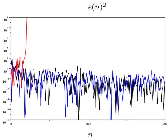
**Fig. 1.** Three runs of LMF with  $M = 10$ , true  $\mathbf{W}_o = [0 \ 0 \ \dots \ 0]^T$ ,  $\mathbf{W}(0) = [1 \ 0 \ \dots \ 0]^T$ ,  $\mu = 0.02$ ,  $\mathbf{X}(n)$  zero-mean Gaussian with covariance equal to  $I$ .
