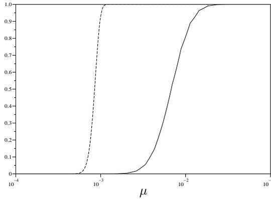
**Fig. 3.** Probability of divergence for LMF, tap-delay line regressors, Gaussian noise,  $M = 100$ ,  $\sigma_0^2 = 0.01$ . Dark curve: observed probability in  $10^5$  runs with 100 time-steps. Broken curve:  $P_d$ .
