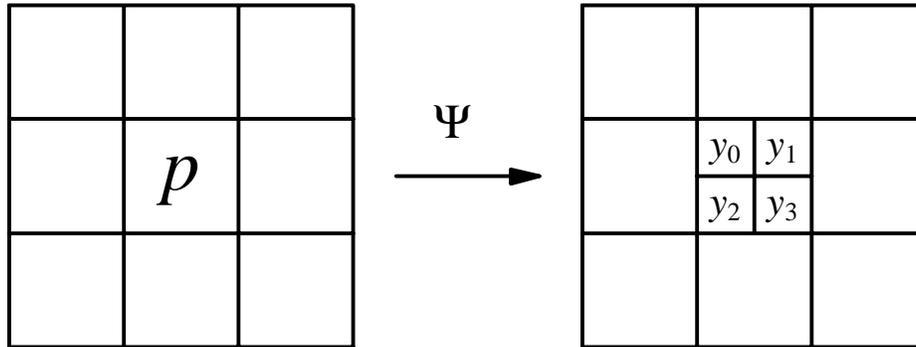
**Figure 3:**  $3 \times 3$  windowed zoom operator with zoom factor  $f=2$ .
