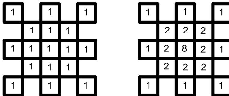
**Figure 4:** Weightless and weighted windows with 17 peepholes.
