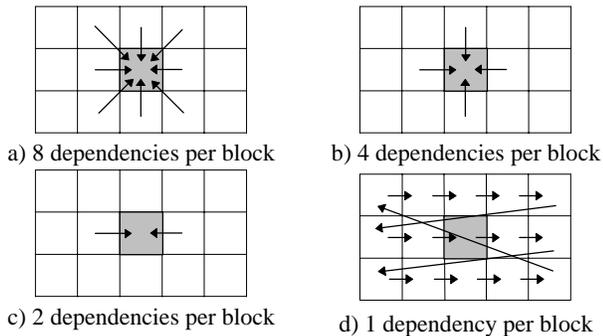
**Fig. 1:** The use of contextual information. To compute the signature of a block  $B$  (shown in gray), the contents of  $B$  and its neighboring blocks are taken into account. Figure (d) shows the chain of dependencies in HBC.
