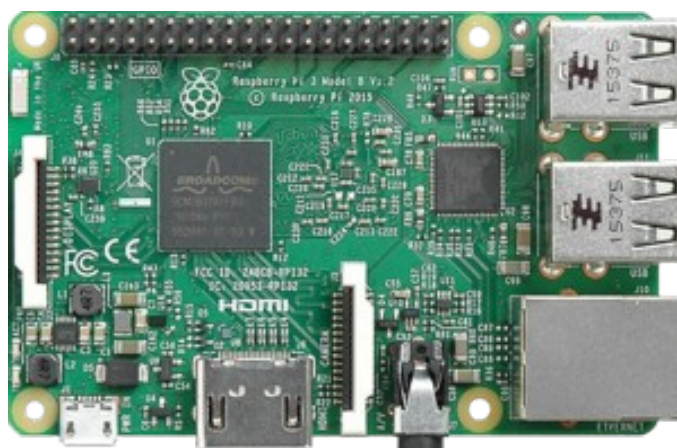
Figura 1: Raspberry Pi 3 Model B (do Wikipedia).
