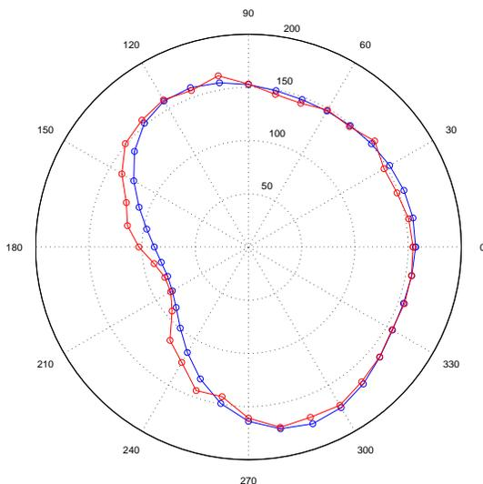
Fig. 3. Single frame of a waist perimeter measuring session. (Red) Raw readings from the sensors. (Blue) Calibrated readings.
