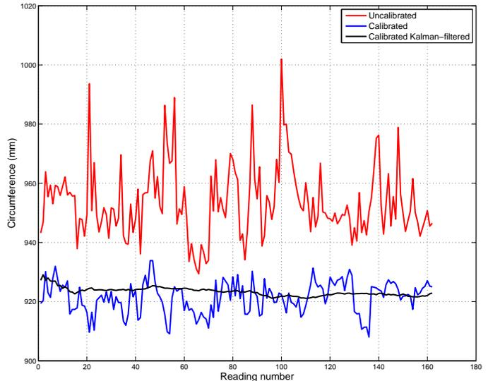
Fig. 4. All 160 measures of the session that measured the perimeter of a man's waist. Uncalibrated measures in red, calibrated measures in blue and Kalman-filtered measures in black.
