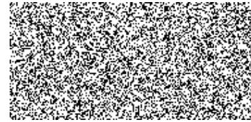
Fig. 5. Part of a 300 × 300 image with 40% random black pixels. It was not possible to reversibly hide 128 bits in this image.
