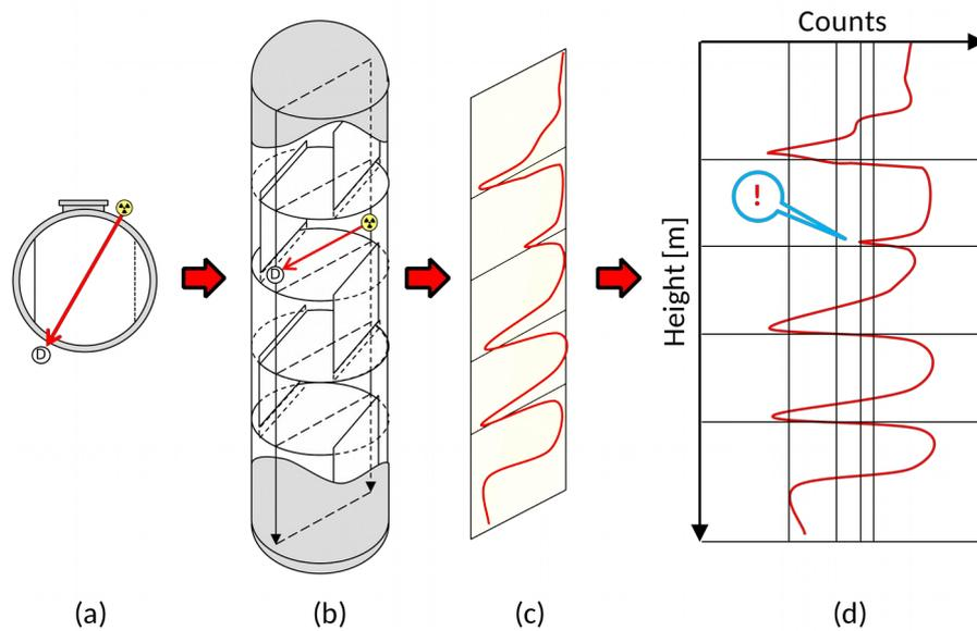
Figure 1: Typical gamma scanning process: job planning (a), field data acquisition (b), plotting (c), reporting and interpreting (d)
