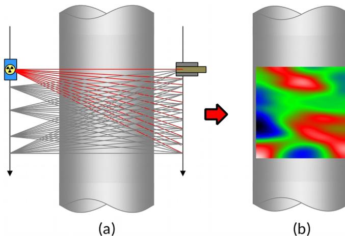
Figure 2: Tomographic Gamma Scan: Movement of source and detector and positioning scheme (a), sketch of an reconstructed image (b).
