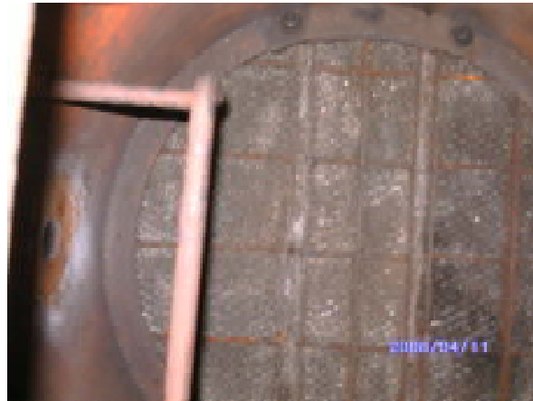
Figure 5. Inspection of the demister pad confirmed that it was saturated with polymer fouling.
