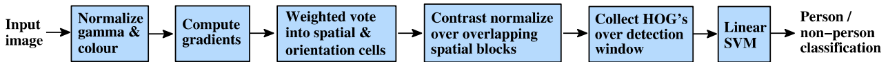
Figure 1. An overview of our feature extraction and object detection chain. The detector window is tiled with a grid of overlapping blocks in which Histogram of Oriented Gradient feature vectors are extracted. The combined vectors are fed to a linear SVM for object/non-object classification. The detection window is scanned across the image at all positions and scales, and conventional non-maximum suppression is run on the output pyramid to detect object instances, but this paper concentrates on the feature extraction process.
