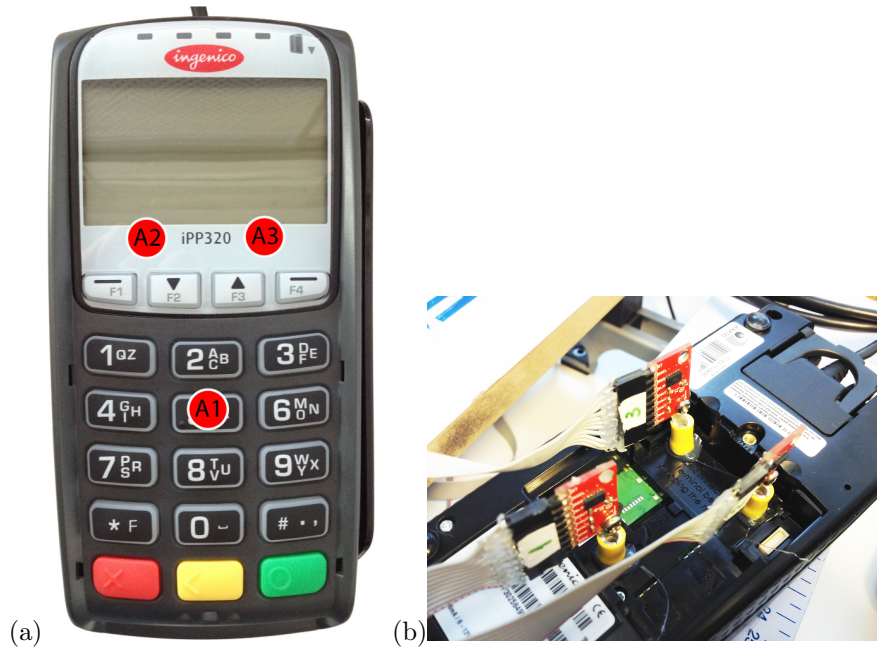
Figure 7: (a) PIN-pad used in the experiment with approximate locations of accelerometers. (b) The bottom view showing the SAM compartment with the implanted accelerometers.
